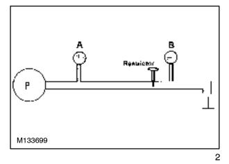
3. When oil in a passage is **fully restricted** from flow (no-flow), the pressure in the passage will build until it reaches the relief valve setting. This relief pressure will be maintained as long as the flow is blocked and the pump is functioning normally. This is true regardless of what component is blocking flow. No flow will create constant pressure in the passage based on the relief valve setting.
