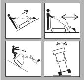
\*\*WARNING Tipover possible. Machine can tip over and crush you.
