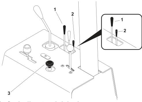
**Note:** Control configuration with rear steer option is shown in main illustration. Control configuration without rear steer is shown in balloon.
