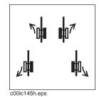
**To steer while moving backward**, pull back and then move to left or right. Drilling unit will gradually turn to left or right.
