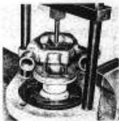
Fig. 9 — Inserting the pulley
