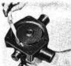
Fig. 10 — Inserting impeller blades
