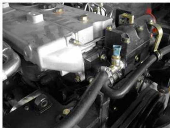
water temperature sensor
