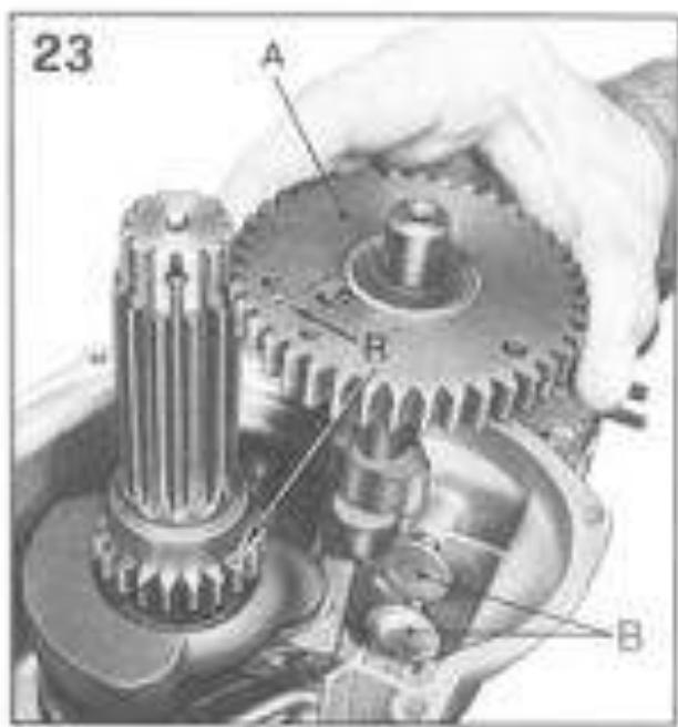
— Notice the timing marks R on the camshaft and the crankshaft A. Mark the lifters in order to reassemble them in the same position. Extract the lifters (fig. 23)
