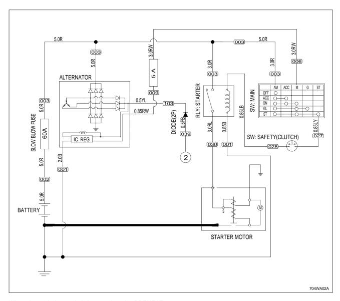
When the main key switch is turned to the PREHEAT position, the terminal AM is connected to the terminal ON and GL. The glow plugs become red-hot. The preheat indicator lamp also lights while preheating.
