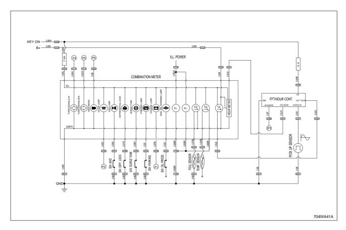
This shows circuit of the Combination meter system.
