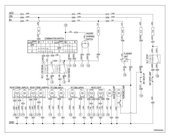
The lighting system consists of combination switch, hazard warning switch, flasher unit, stop lamp relay, stop switch, head lights, turn signal lamps, tail lamps and stop lamps.
